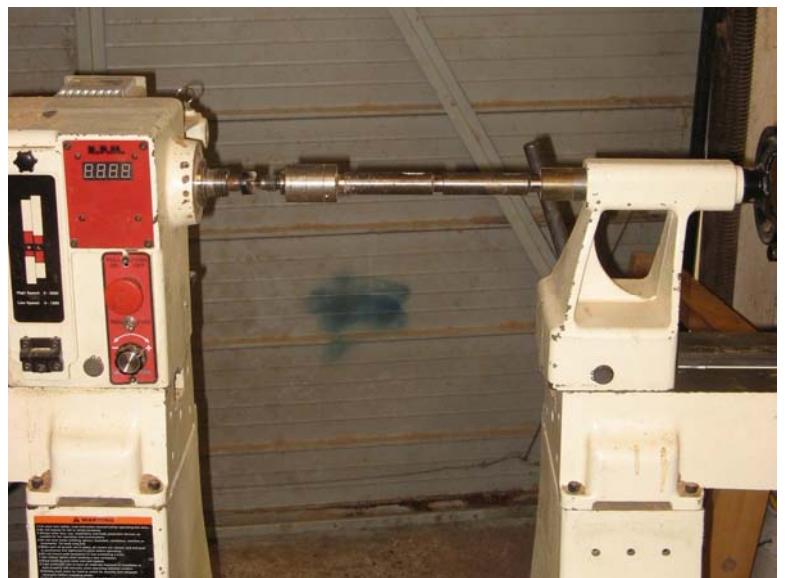
Picture 3 – Two lathes operating as one
